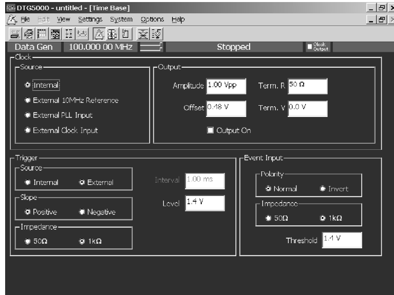
Figure 1-42: Time Base window (Data Generator mode)
